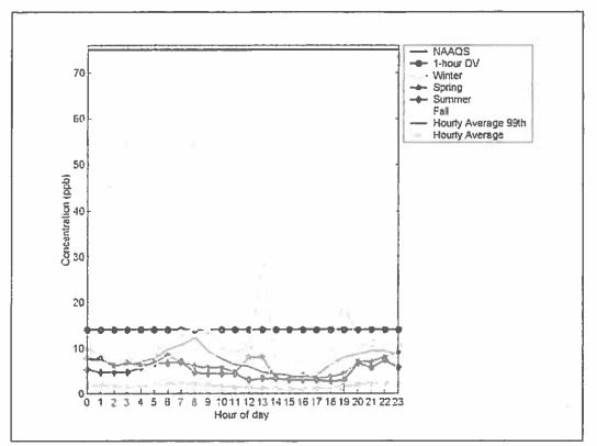
Figure 3. SO<sub>2</sub> monitored concentrations for various averaging times.
