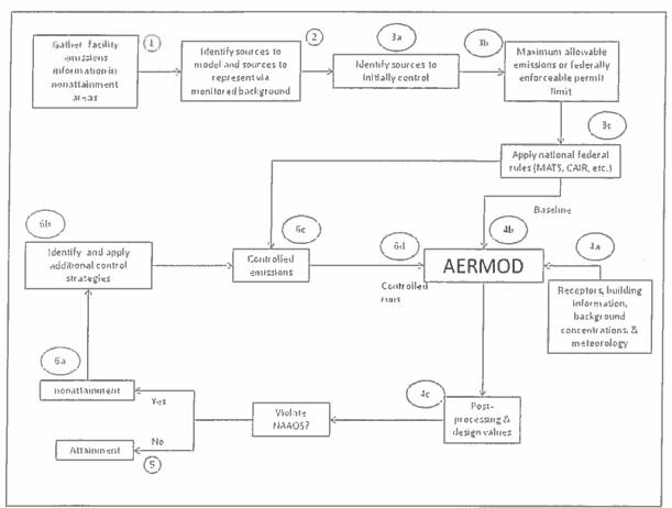
Figure 2. Flowchart of SO<sub>2</sub> Modeling Framework for SIP Demonstration.
